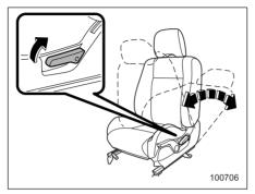
Pull the reclining lever up and adjust the seatback to the desired position. Then release the lever and make sure the seatback is securely locked into place. The seatback placed in a reclined position can spring back upward with force when
