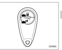
CLOCK/ARM button Press to Lock all doors. Press and Hold to activate panic alarm.
