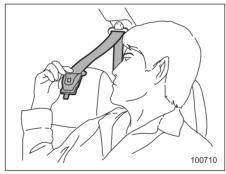
1. Remove the tongue plate from the belt holder located under the right rear quarter glass and pull out the seatbelt slowly.
