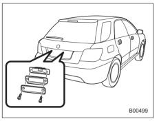
1. Remove the mounting screws using a Phillips screwdriver.
