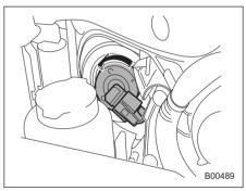
1. Remove the bulb from the headlight assembly by turning it counterclockwise.
