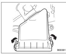
1. Unsnap the two clamps holding the air cleaner case cover.
