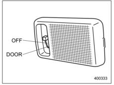
**DOOR:**The light comes on only when the rear liftgate is opened. **OFF:** The light stays off.
