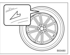
Unidirectional tires: Some tires have a specified direction of rotation. A tire of this type has an arrow or other mark on its side wall to indicate the direction of rotation. Install it so that the direction of rotation is correct when the vehicle is driven forward.
