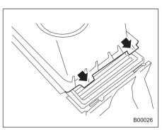
4. To install the air cleaner case cover, insert the two projections on the air cleaner case cover into the slits on the air cleaner case and then snap the two clamps on the air cleaner case cover.
