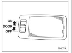
The dome light switch has three positions:
