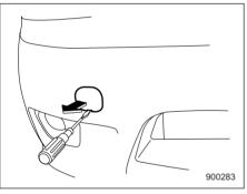
2. Insert a flat-head screwdriver into the slot on the towing hook cover, then use it to pry the cover upward.
