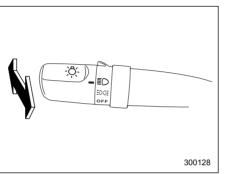
To change from low beam to high beam, push the turn signal lever forward. When the headlights are on high beam, the high beam indicator light "  $\equiv \bigcirc$  " on the instrument panel is also on.
