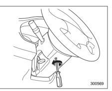
2. Remove the cover under the steering column using a Phillips screwdriver.
