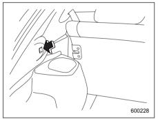
2. Insert the projections located on the both ends of the sleeve into the recesses of the retainers.
