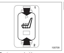
Front passenger's side 1) HI – Rapid heating 2) LO – Normal heating
