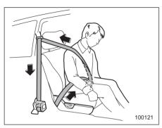
The driver's and front passenger's seatbelts have a seatbelt pretensioner. The seatbelt pretensioners are designed to be activated in the event of an accident involving a moderate to severe frontal collision.
