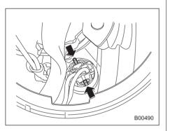
3. Hold the end of the parking light and remove the parking light.
