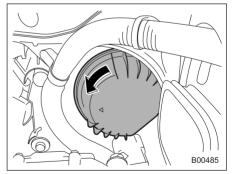
2. Remove the bulb cover by turning it counterclockwise.
