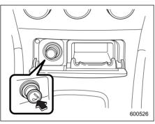
The cigarette lighter operates only when the ignition switch is in the "ON" and "ACC" positions.
