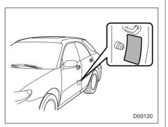
The load capacity of your vehicle is determined by weight, not by available cargo space. The maximum load you can carry in your vehicle is shown on the vehicle label attached to the driver's side door pillar. It includes the total weight of driver and all passengers and their belongings, any optional equipment such as a trailer hitch, roof rack or bike carrier, etc., and the tongue load of a trailer.
