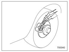
The disc brake pad wear warning indicators on the disc brakes give a warning noise when the brake pads are worn. If a squeaking or scraping noise is heard from the disc brakes while braking, immediately have your vehicle checked by your Saab dealer.
