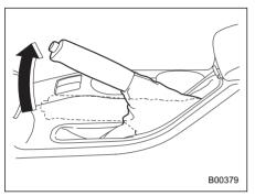
Check the parking brake stroke according to the maintenance schedule in the "Saab Warranty and Service Record Booklet". When the parking brake is properly adjusted, braking power is fully applied by pulling the lever up seven to eight notches gently but firmly (approximately 44 lbs [196 N, 20 kg]). If the parking brake lever stroke is not within the specified range, have the brake system checked and adjusted at your Saab dealer.
