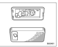
1. Remove the lens by prying the edge of the lens with a flat-head screwdriver.
