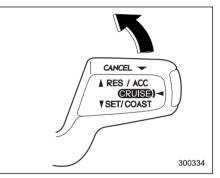
Push the control lever upward in the "RES/ACC" direction and hold it until the vehicle reaches the desired speed. Then, release the control lever. The vehicle speed at that moment will be memorized and treated as the new set speed.
