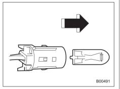
4. Pull the bulb out of the socket. Install a new bulb.
