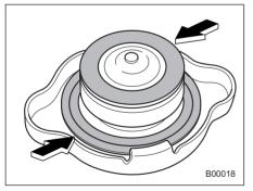
7. Put the radiator cap back on and tighten firmly. At this time, make sure that the rubber gasket in the radiator cap is correctly in place.
