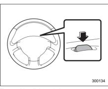
The parking light switch operates regardless of the ignition switch position.
