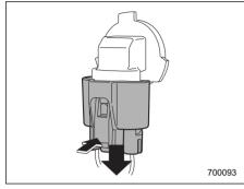
2. Remove the electrical connector from the bulb.
