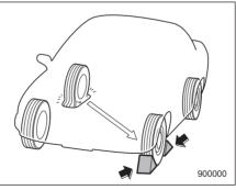
4. Put wheel blocks at the front and rear of the tire diagonally opposite the flat tire.
