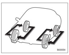
Tire wear varies from wheel to wheel. To maximize the life of each tire and ensure that the tires wear uniformly, it is best to rotate the tires every 7,500 miles (12,500 km). Rotating the tires involves switching the front and rear tires on the right-hand side of the vehicle and similarly switching the front and rear tires on the left-hand side of the vehicle. (Each tire must be kept on its original side of the vehicle.)
