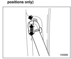
The shoulder belt anchor height should be adjusted to the position best suited for you. To adjust the anchor height, push the release button and slide the anchor up or down. Pull down on the anchor to make sure that it is locked in place.
