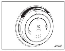
This dial is used to set the desired interior temperature. With the dial set to your desired temperature, the system automatically adjusts the temperature of air supplied from the outlets such that the desired temperature is achieved and maintained. If the dial is turned fully counterclockwise, the system gives maximum cooling performance. If the dial is turned fully clockwise, the system gives maximum heating performance.
