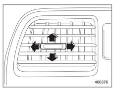
Move the tab up and down or right and left to adjust the air flow direction.
