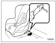
2. While following the instructions supplied by the child restraint system manufacturer, connect the lower hooks onto the lower anchorages located at " S" marks on the bottom of the rear seatback. When the hooks are connected, make sure the adjacent seatbelts are not caught.
