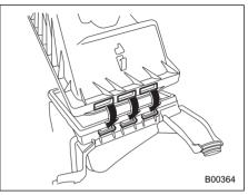
5. To install the air cleaner case cover, insert the three projections on the air cleaner case into the slits on the air cleaner case cover and then snap the two clamps on the air cleaner case cover.
