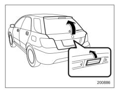
The rear liftgate can be locked and unlocked using either the keyless entry system or the power door locking switches.
