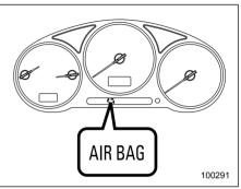
A diagnostic system continually monitors the readiness of the SRS airbag system (including front seatbelt pretensioners) while the vehicle is being driven. The SRS airbag system warning light "AIRBAG" will show normal system operation by lighting for approximately 6 seconds when the ignition switch is turned to the "ON" position.
