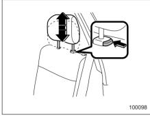
To raise the head restraint, pull it up. To lower it, push the head restraint down while depressing the release button on the top of the seatback.
