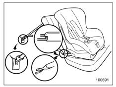
Some types of child restraint systems can be installed on the rear seat of your vehicle without use of the seatbelts. Such child restraint systems are secured to the designated anchorages provided on the vehicle body. The lower and tether anchorag-
