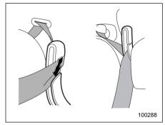
2. After drawing out the seatbelt, pass it through the belt guide as follows: First insert one edge of the belt into the open gap in the comfort guide; then slide the rest of the belt in, so that the whole belt fits inside.
