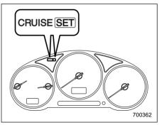
At this time, the " (SET) " indicator light is illuminated in the instrument cluster.
