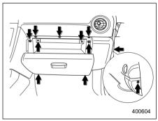
6. Connect the connector, and reinstall the glove box.
