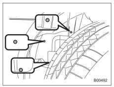
2. Undo the three clips at the bottom of the undercover beside the front-left wheel.
