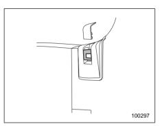
2. (For both window-side seating positions) Remove the cap from the anchor fitting cover by prying it with a screwdriver.
