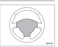
To sound the horn, push the horn pad.
