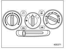
This setting allows you to direct air of different temperatures from the instrument panel and foot outlets. The air from the foot outlets is slightly warmer than from the instrument panel outlets.
