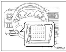
One is located under the instrument panel behind the coin tray on the driver's seat side.
