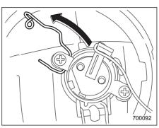
3. Push the retainer spring in the direction of the arrow to remove it from the hook.
