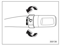
When the wiper switch is in the "  $\sqrt{2}$  " position, turn the dial to adjust the operating interval of the wiper.
