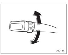
When the headlight switch is in the " $\exists c D a \equiv 0$ " or " $\equiv c D$ " position, you can adjust brightness of the instrument panel illumination for better visibility.
