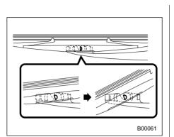
2. Turn the wiper blade assembly counterclockwise.
