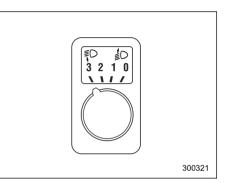
On cars so equipped, the low beam headlights are the High-Intensity Discharge type. The HID headlights generate more light than conventional halogen headlights. Therefore a driver of an oncoming vehicle may experience too much glare when your headlight beam height adjustment is high due to the vehicle carrying heavy load.
