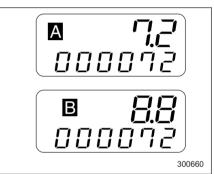
The trip meter shows the distance that the vehicle has been driven since you last set it to zero.
