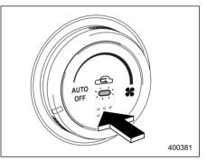
**ON position (Recirculation):** Interior air is recirculated inside the vehicle. Push the air inlet selection button to the ON position for fast cooling with the air conditioner or when driving on a dusty road. The indicator light will come on.
