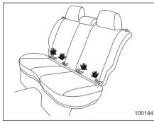
The lower anchorages (bars) are used for installing a child restraint system only on the rear seat window-side seating positions. For each window-side seating position, two lower anchorages are provided. Each lower anchorage is located where the seat cushion meets the seatback.
