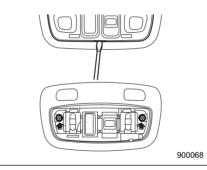
2. Remove the map light lens by prying the edge of the lens using a flat-head screwdriver.
