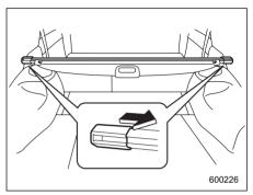
Pull either sleeve on the end of the cover housing to shorten the cover's length.
