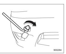
4. Tighten the towing hook securely using the wheel nut wrench.
