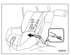
3. [If your child restraint system is of a flexible attachment type (which uses tether belts to connect the child restraint system properly to the lower anchorages)] While pushing the child restraint into the seat cushion, pull both left and right lower tether belts up to secure the child restraint system firmly by taking up the slack in the belt.
