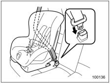
1. Place the child restraint system in the rear seating position.
