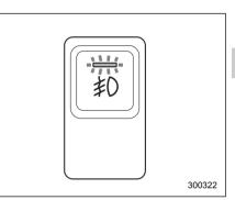
The front fog lights operate only when the headlights are on low beam. Push the front fog light button to turn the front fog lights on.
