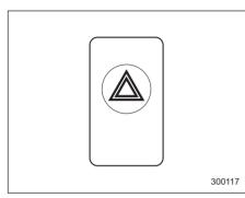
The hazard warning flasher is used to warn other drivers when you have to park your vehicle under emergency conditions. The hazard warning flasher works with the ignition switch in any position.
