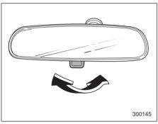
The inside mirror has a day and night position. Pull the tab at the bottom of the mirror toward you for the night position. Push it away for the day position. The night position reduces glare from headlights.
