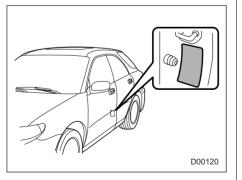
Check the tire pressures when the tires are cold. Use a pressure gauge to adjust the tire pressures to the values shown on the tire label. The tire label is located on the door pillar on the driver's side.
