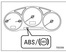
The ABS warning light comes on when the ignition switch is turned to the "ON" position and goes out after approximately two seconds.
