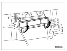
2. Unhook the hooks of the air filter cover and remove the cover.
