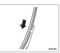
4. Align the claws of the plastic support with the grooves in the blade rubber assembly, then slide the blade rubber assembly into place.
