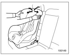
5. Before seating a child in the child restraint system, try to move seat back and forth and right and left to verify that it is held securely in position.
