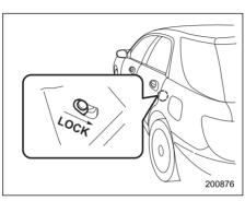
Each rear door has a child safety lock that prevents the doors from being opened even if the inside door handle is pulled. When the child safety lock lever is in the lock position, the door cannot be opened from inside regardless of the position of the inner door handle lock lever. The door can only be opened from the outside.
