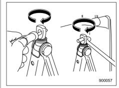
After placing the jack in its storage location, turn the jackscrew clockwise by hand until it becomes too hard to turn. Then, tighten it by an additional 1/4 - 1/3 of a turn using a screwdriver or the jack handle. Unless the jack is properly secured, it may rattle while the vehicle is moving.
