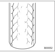
Ride comfort is poor. Also, the tire magnifies the effects of road-surface bumps and dips, possibly resulting in vehicle damage.
