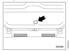
Remove the access cover at the bottom-center of the rear liftgate trim.
