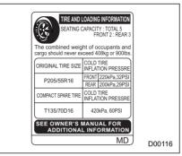
The vehicle label shows original tire size, recommended cold tire inflation pressure on each tire at maximum loaded vehicle weight, seating capacity and loading information.
