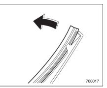
1. Pull out the end of the blade rubber assembly to unlock it from the plastic support.
