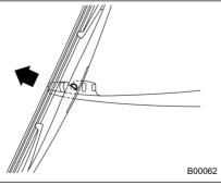
3. Pull the wiper blade assembly toward you to remove it from the wiper arm.
