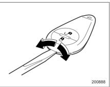
1. Open the transmitter case using a flathead screwdriver.
