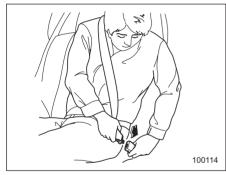
4. Insert the center seatbelt tongue plate in the center seatbelt buckle marked "CENTER" on the left-hand side until it clicks.
