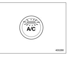
The air conditioner operates only when the engine is running.
