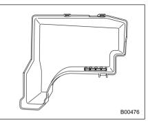
The spare fuses are stored in the main fuse box cover in the engine compartment.
