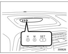
To set the hour, press the "H" button. To set the minutes, press the "M" button. To reset the minutes to "00" with a radio time signal, push the "SET" button.
